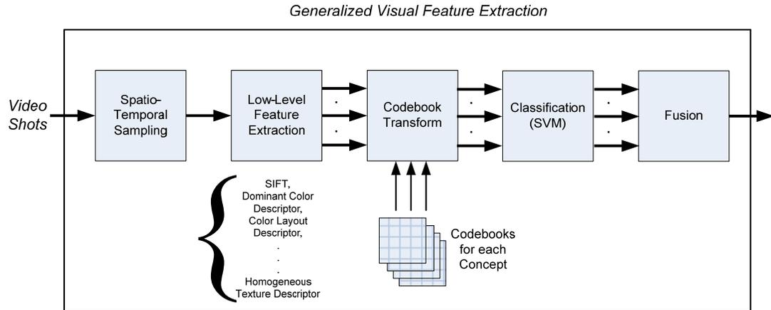
**Figure 4: Generalized Visual Feature Extraction block diagram.**
